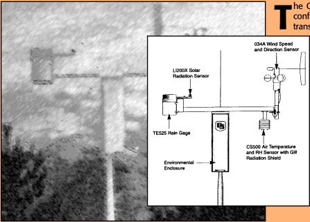
he Campbell Scientific ET101 and ET106 are preconfigured stations that calculate potential evapotranspiration (ETo) using a turf grass reference. The
