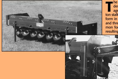
he AMADAS **CSP01 Cotton Stalk Puller/Chopper** is designed to streamline post-harvest cotton stalk management and field preparation. Pulling up an entire cotton stalk and chopping it into small pieces, the CSP01 can perform in a single pass what previously took several machines and three to five passes. Operating at 8 to 12 mph, it is common for this four-row machine to cover 100 acres per day, resulting in time and cost savings. Other benefits include
