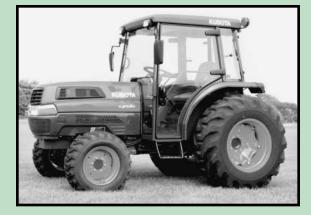
ECU, it controls operation of the solenoid and proportional reducing valves for effortless one-touch shifting of the proven Glide Shift Transmission. All of this plus many more upgrades were accomplished while maintaining a price competitive with traditional compact tractors.
