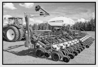
7571-liter (2000-gallon) nurse tank. In addition to the new frame, markers, and fertilizer system improvements over the previous models, the 1790 offers the increased productivity of the Central Commodity System (CCS) Seed Delivery and the new Pro-Series Row Unit.
