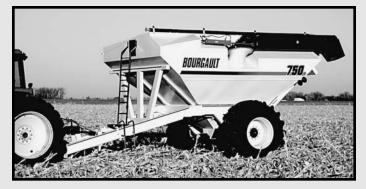
inated. The turret auger's position can be hydraulically controlled from the tractor allowing the flow of grain from the cart to be directed to the desired location in the truck box or trailer. A high-clearance frame design provides access to a gravity chute which allows the contents of the 750 Smart Cart to be drained into a pit or auger systems.
