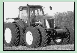
option and front duals are available with any axle on the larger two models. Increased hydraulic flow up to 257.4 liters (68 gallons) per minute is available with the New Holland exclusive MegaFlow<sup>™</sup> system. The cab interior volume is increased to 109.5 cubic feet (3.1cubic meters), increasing operator comfort and visibility.
