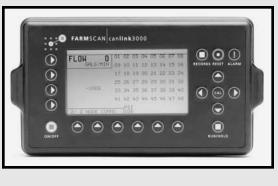
The Farmscan Canlink 3000 Center Pivot Irrigation Controller converts existing pivot irrigation systems into site-specific, variable-rate water application systems. The system enables area specific watering under center pivots by cycling sprinklers on and off according to a predetermined prescription and guided by GPS positioning. Additionally, it
