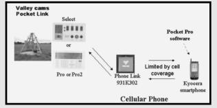
travel, position in the field, water on or off, pivot or linear on/off, and auxiliary relay diagnostics. The operator may control start or stop, select the direction of travel, start or stop the water (if equipped) change endgun settings, auxiliary relays on or off, and set service road stop. Specific items monitored and controlled are dependent on the functions supported by the control panel.
