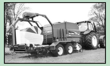
in only 6 to 8 additional seconds. Then formation of a new bale can begin. The compact design allows excellent maneuverability in small fields with tight corners and is engineered to assure proper transfer of the bale, even on sloping ground.
