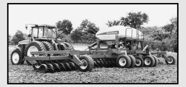
onto the tool reduces overall cost and horsepower requirements to make the 1690CCS more economical. Large central tanks, wide widths, and fast operating speeds mean increased productivity. Standard features include in-cab rate adjustment, accurate seed counting monitor, low level bin sensor, half-width disconnect, and choice of three metering wheels. Optional features include rear auxiliary hydraulic couplers and platformmounted fill lights.
