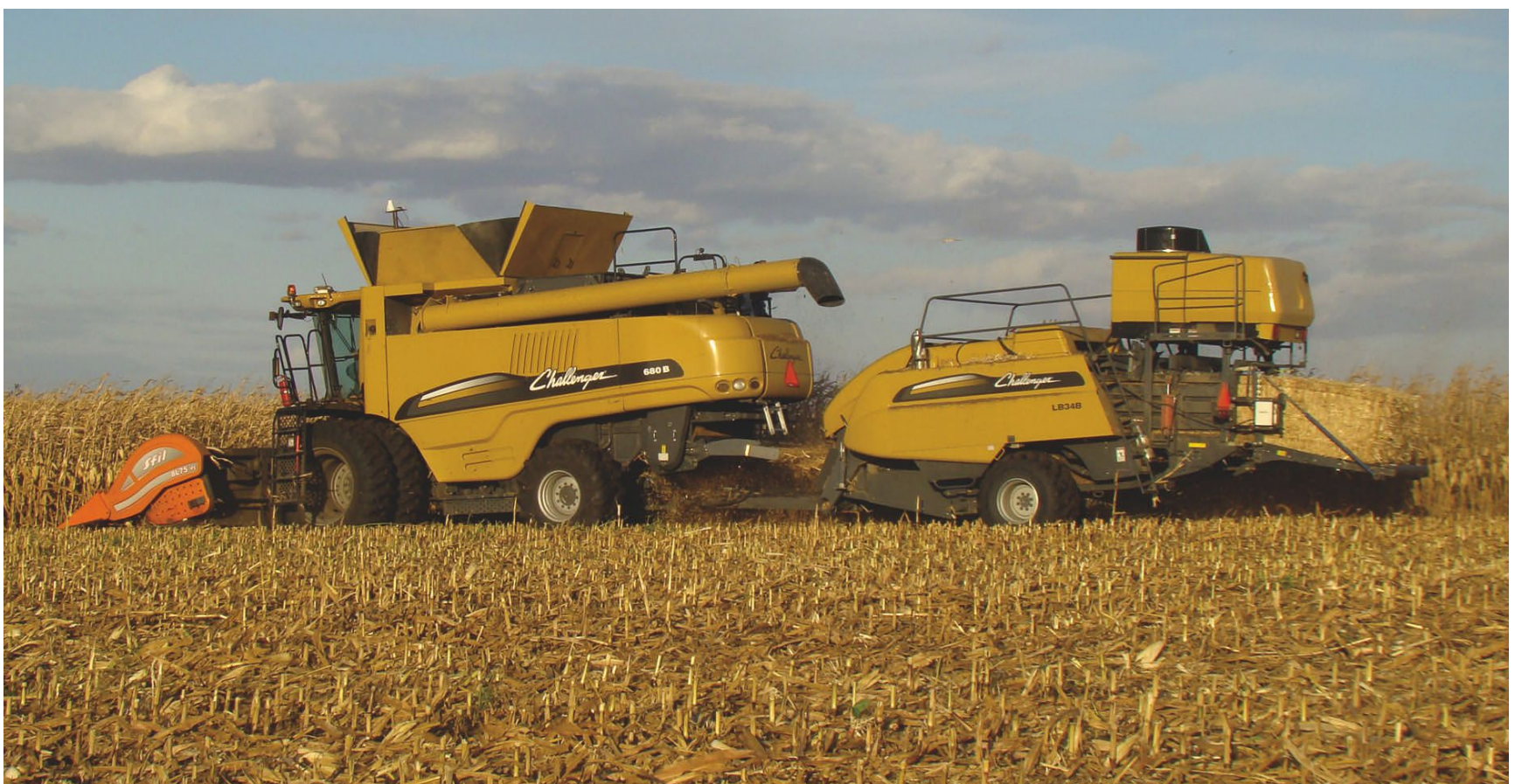
CAN Bus information can enable detailed assessment of new machinery systems, such as single-pass harvesting of corn grain and stover.
