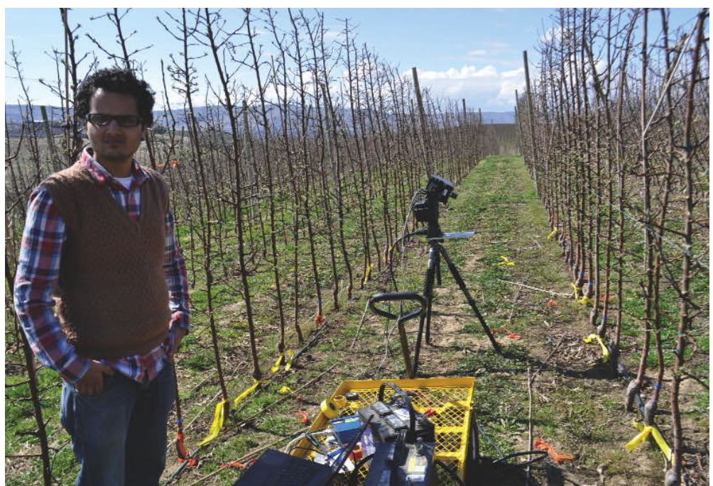
Co-author Karkee stands amidst hyperspectral and 3D cameras scanning apple trees in a mechanization-friendly tall-spindle orchard. Photo courtesy of Allan Bros., Inc., Prosser, Wash., USA.
