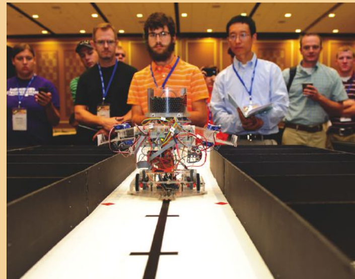
The 2012 Robotics Competition required the design of an automated machine to deposit "feed" into a series of bins.
