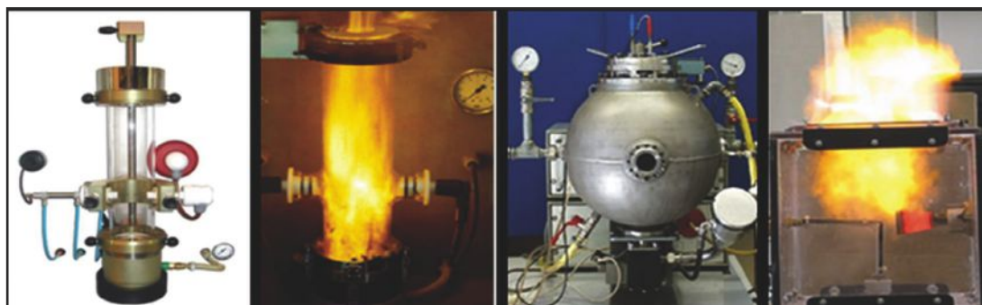
Figure 1. (left to right) The Hartman tube used by SCE, the Hartman tube in operation, the 20 L spherical chamber specified by ASTM, and the 28.3 L (1 ft 3 ) CAAQES chamber.
