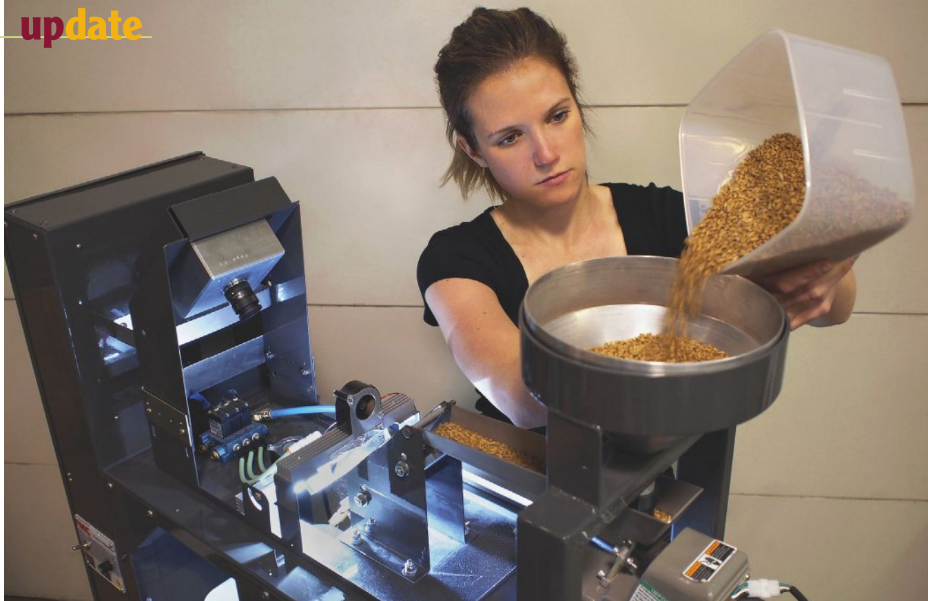
Biological science aide Anne Berry puts wheat in the hopper of a color-image sorter. The camera behind her captures a color image of each kernel as it falls off the end of the chute. The kernels are then sorted based on visual features and deposited into either of two separate buckets at the base of the sorter. This fast, accurate, and economical seed sorter is proving popular with a variety of users. Photo by Thomas Pearson.
