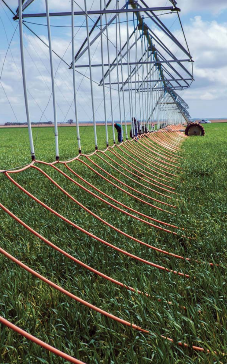
The Dragon-Line Precision Mobile Drip Irrigation (PMDI) system reduces water use by an estimated 20% to 50%.
