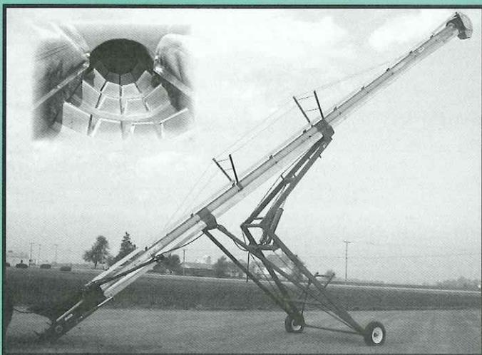
(10-in.) galvanized tube and has a completely enclosed belt return. It comes in lengths from 5.8 to 21.9 m (19 to 72 ft) with cable or hydraulic scissors-lift system. Electric, PTO, and hydraulic drive options are available.
