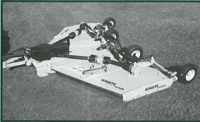
Rilsan coating for ease of telescoping. The FX520 features walking axles for increased ground following capabilities.
